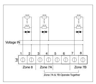
Figure C-3 Typical Signal Device Wiring—Terminal Block P1
